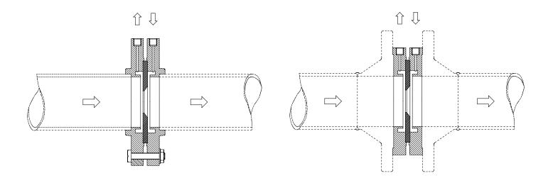
Calibrated element with ring chambers fitting pipes from DN50 to DN400 included
