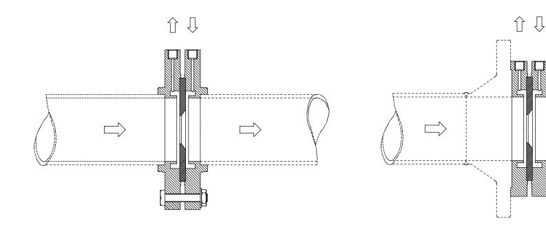
Calibrated element with ring chambers fitting pipes from DN50 to DN400 included
